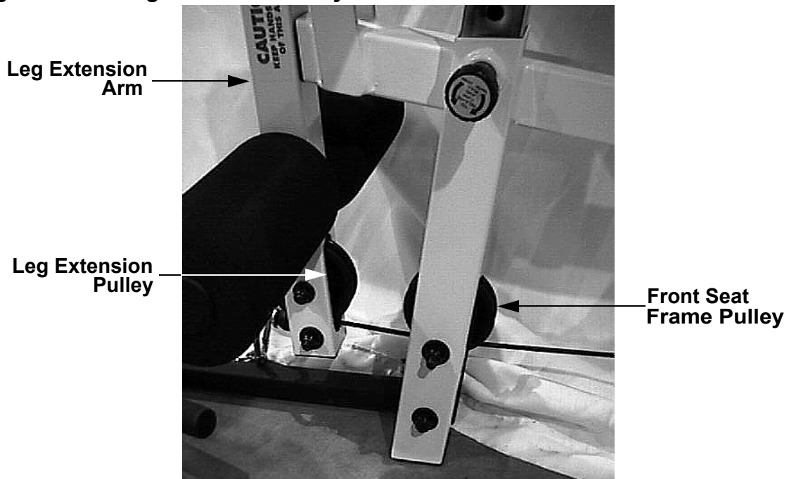
Diagram 4.36 - Leg Extension Pulleys
