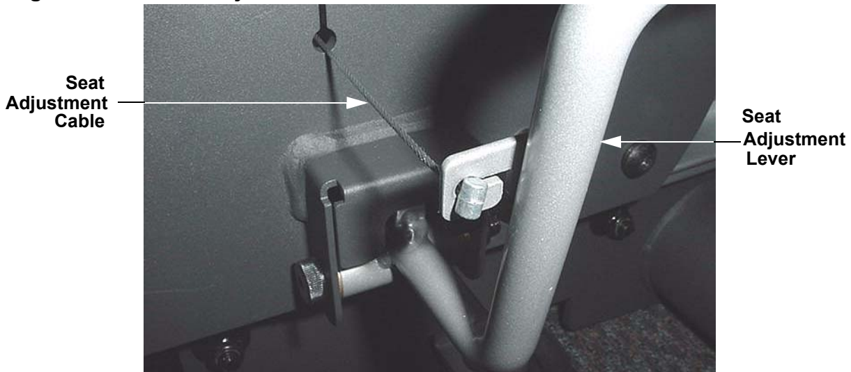
Diagram 4.62 - Seat Adjustment Lever
